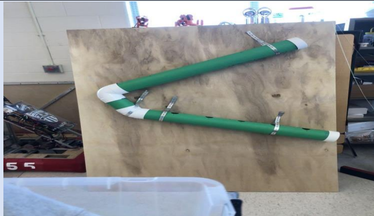
Figure C3: Attaching PVC to the Board
