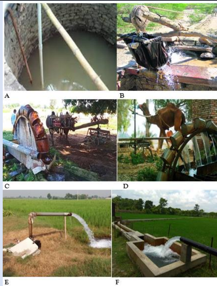
Figure 1: In rural areas of India, water from dug wells (Figures A-D) and bore-wells (Figures E and F) is used for irrigation of agriculture by adopting traditional and advanced methods, respectively.
