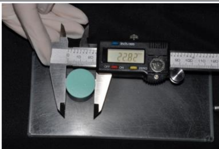
Figure 4: Specimen being measured with digital caliper in circumference
