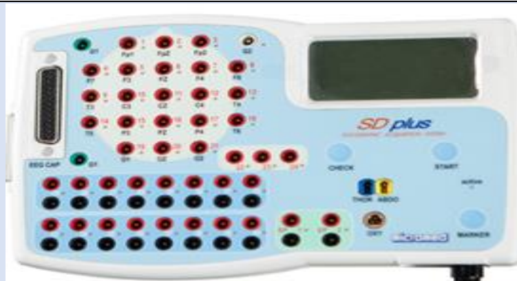
Figure 3: 29-channel quantitative electroencephalography (QEEG)
